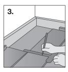
Cut and position to complete the first row. Joints should be staggered. If the off-cut is between 300mm - 900mm it can be used to start the next row; otherwise, halve a board.
