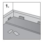
Lay the next board end-on, placing the short tongue of the second board into the long tongue of the first at a 30° angle. Lower the board and lock into place. Lay more boards in the same way until you reach the end of the row, where you will probably have to cut a board to make it fit.
